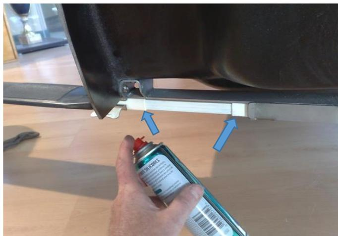
*The assembly of the rear fiberglass axles is as shown in the pictures below. There is a spring-metal piece on each axle, (it is a safety system in case of shock). Put some silicone spray or any lubricant at the places indicated in the picture above. If the white rubber sleeves are too dry, it will be hard to mount the axles.*
